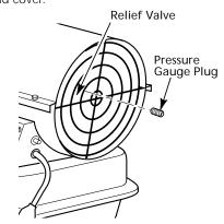
Figure 9 - Pressure Gauge Plug Removal
